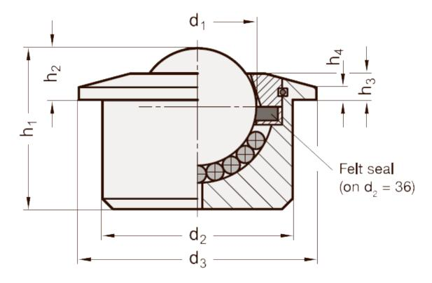
$$\begin{array}{lll} d1 & = 30.1 \\ d2 + / -0.08 & = 45 \\ d3 & = 55 \\ h1 + / -0.3 & = 36.8 \\ h2 + / -0.3 & = 13.8 \\ h3 + / -0.3 & = 7 \\ h4 & = 4.5 \\ Max load (N) = 2000 \end{array}$$
